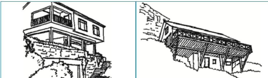
Buildings on stilts or open columns are uncharacteristic in heritage areas.
