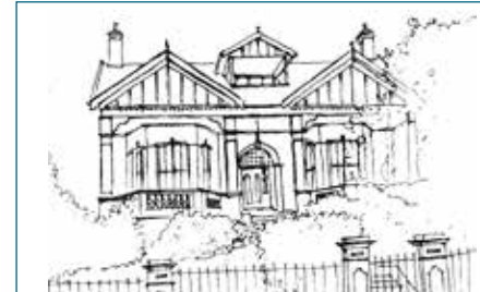
New dormer window positioned to reinforce strong symmetry of house, and detailed sympathetically.
