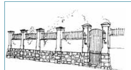
To increase the height of the original low wall, columns were extended, more brick courses added, and the column heads and fencing reused.
