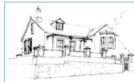
Roof space converted into loft room, and well-scaled dormer inserted.
