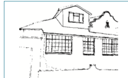
Poorly scaled and designed dormer addition.
