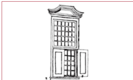
Unobtrusive internal dark burglar bars in keeping with the glazing pattern of the window.
