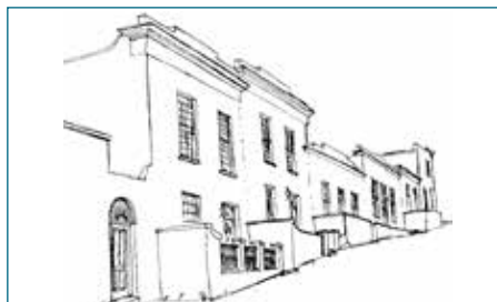
Typical flat roofs with parapet walls in the Bo-Kaap.
