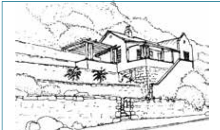
Interlocking-block retaining walls are visually inappropriate. Rather use natural stone terrace walls and planting.
